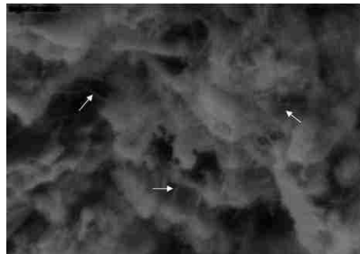
Figure 23. SEM image of 0.03% CNT/cement specimen [8]
