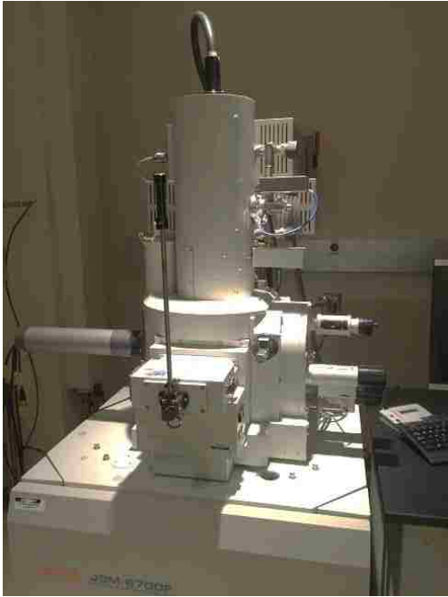
Figure 57. FESEM scanning electron microscope (JEOL) JSM-6700F
