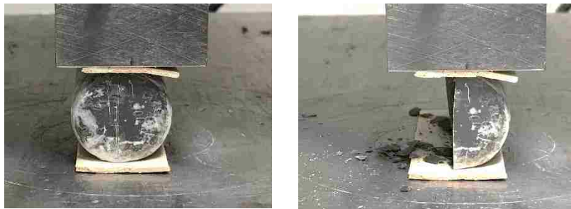
Figure 71. Cement mortar sample failure mechanism in splitting tensile test (sudden cement mortar failure)
