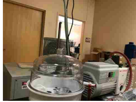
Figure 54. a) Fractured specimen b) drying in desiccator
