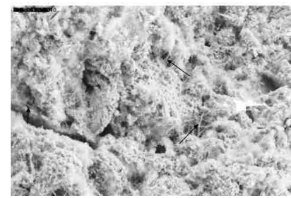
Figure 24. SEM image of dispersed MWCNTs in water [26]
