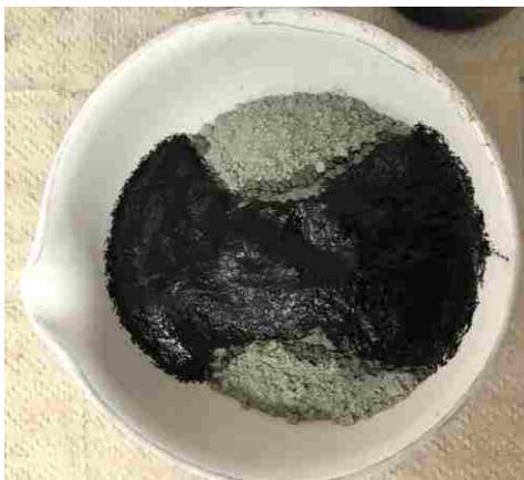
Figure 51. Mixing dispersed carbon nanotubes with cement
