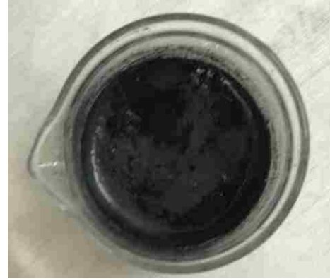
Figure 50. Dispersed multi-walled carbon nanotubes after an hour sonication at amplitude of 30%
