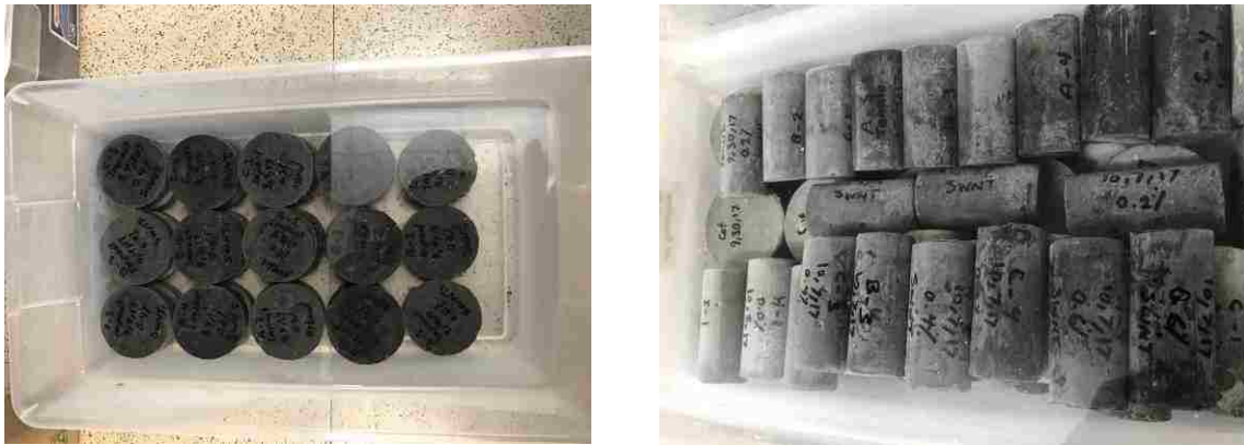
Figure 53. Impact and tensile cementitious nanocomposite specimen curing
