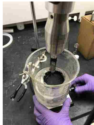
Figure 49. Melted ice bath and application of new ice bath
