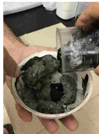
Figure 51. Mixing dispersed carbon nanotubes with cement
