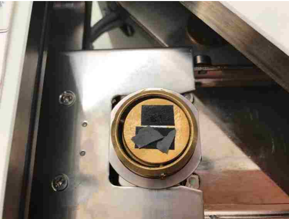
Figure 58. Placing sample for scanning electron microscope
