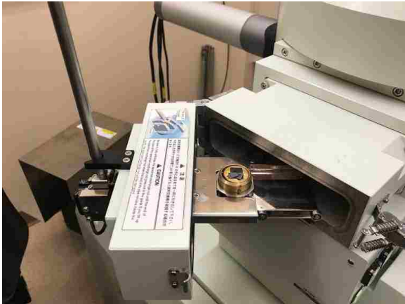
Figure 58. Placing sample for scanning electron microscope
