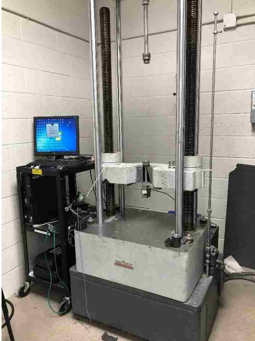
Figure 69. Load cell with 5,000lbf capacity for nanocomposites incorporating hybrid CNTs
