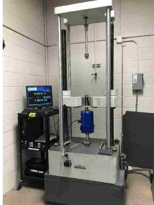
Figure 70. Load cell with 5000lbf capacity for nanocomposites incorporating MWCNTs and SWCNTs
