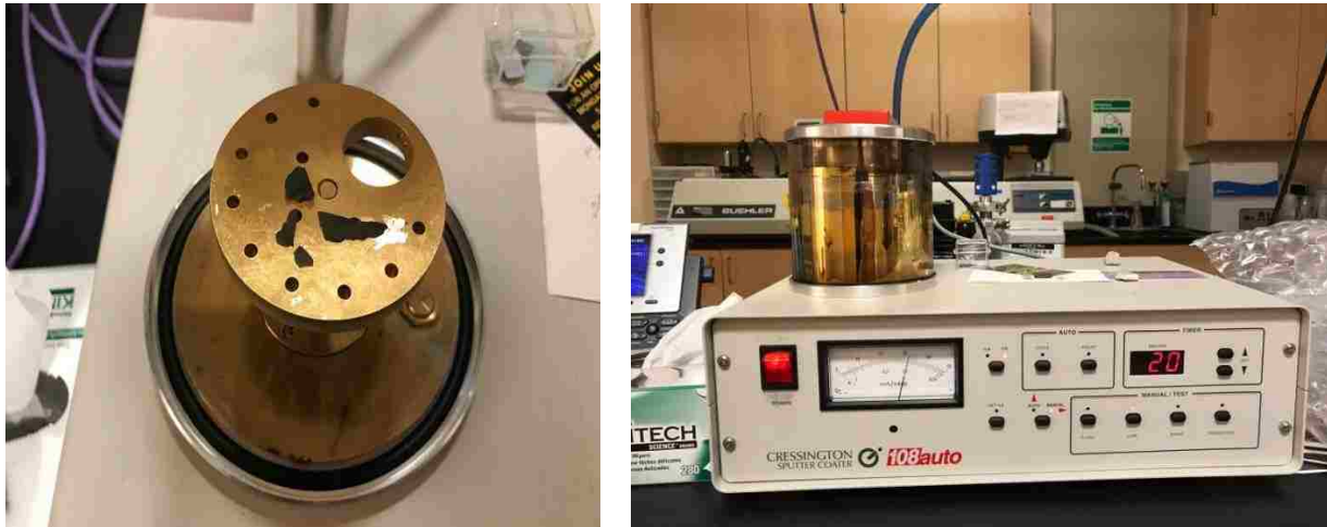
Figure 56. Coating the sample with gold for better electron discharge (Cressington 108 auto sputter coater)
