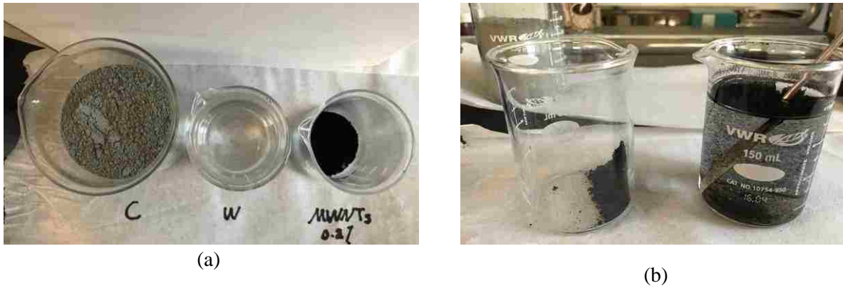
Figure 44. (a) Cement, water, and multi-walled carbon nanotubes were scaled (b) MWCNTs were gradually added to water
