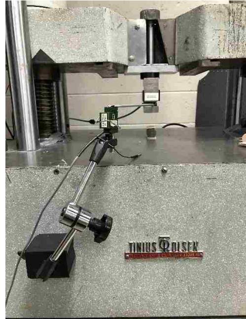
Figure 68. Schematic test setup for splitting-tensile test and specimen test set up before applying load
